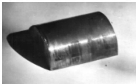
Picture 2: Section of pin of the high pressure cylinder
